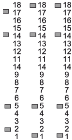
Fig. 171: Encoding for I/O modules (120 VAC / 230 VAC)
